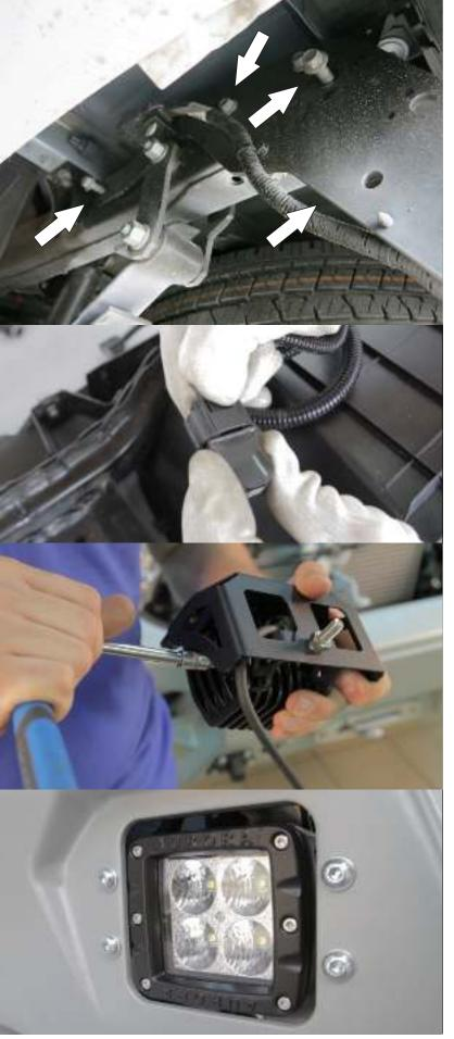
1. Unscrew tension bolts of the standard under-run bar the left and right of the vehicle frame.
