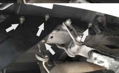
7. Install the bracket onto completed bolts. Secure it using standard tension bolts of the bumper.
