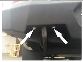
8. Install the bumper facia (pos. 1) onto the bracket and secure it in the towing eye area using screws M10x30 (pos. 7) and washers 10 (pos. 9).
