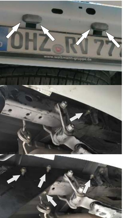
5. Unscrew self-tapping screws of the license plate lamps.
