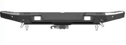
11. Install the bumper facia onto the bracket and screw it in the 4 screws M10x30 and wahsers M10
