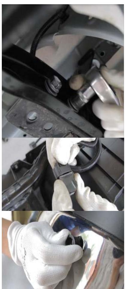
1. Unscrew tension bolts of the standard bumper the left and right of the vehicle frame.
