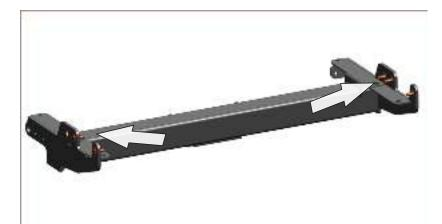
11. Install bumper bracket on the car frame. Fasten with bolts M12x24x1,25 with washers M12x24.
