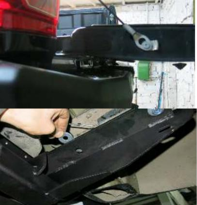
**14. Carefully** open the vehicle board. Check for the clearance between the bumper and board which should be 20 mm at least.
