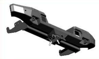
13. Instal the socket bracket on the towing bar bracket and screw with 2 bolts M12x1,25x30 and washers M12x24 on several turns.
