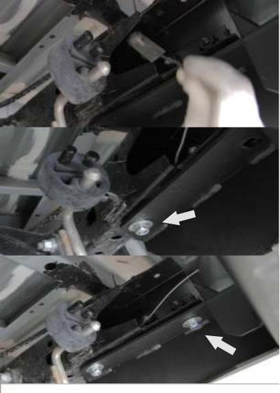
9. Put insert pin M10 (17) into the car frame. Screw on nut M10 and washer M10x30.
