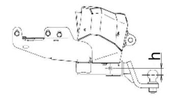
Towing of the trailer which is incompliant with specified requirements may result in damage to tow bar or bumper.
