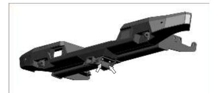
12. Instal the towing bar bracket on the car and screw with 2 bolts M12x1,25x30 and washers M12x24 on several turns.
