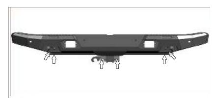
15. To align the bumper facing in relation to the vehicle body in order to achieve the equal clearance on the left and right.
