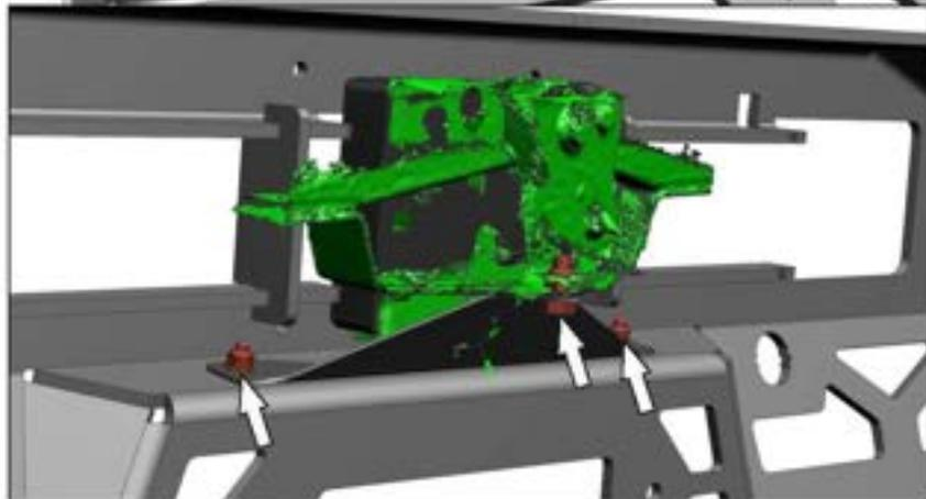
30. Install the radar and bracket №2 (15) in bumper, using screws M6x25 (G), washers 6 (M), nuts M6 (J), bolt M8x20 (B), washers 8 (O), nut M8 (K), as shown.
