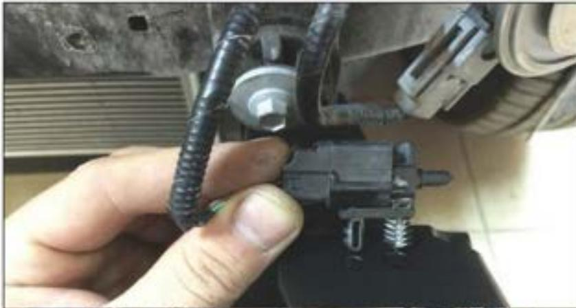
25. Fix temperature sensor to the bracket.
