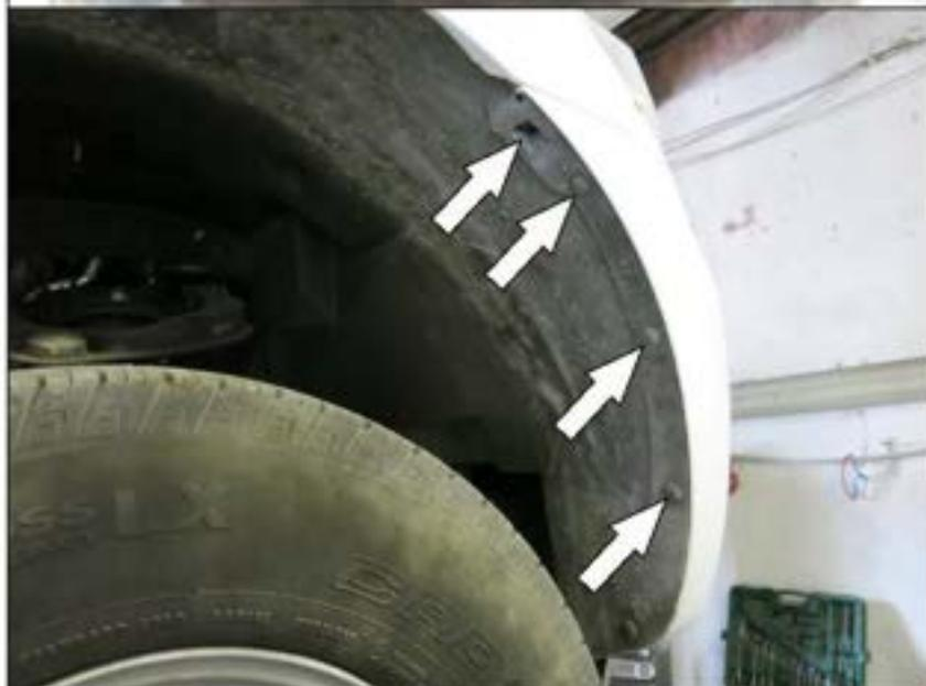
3. Remove 3 screws from inside of the fenders on each side of the vehicle.
