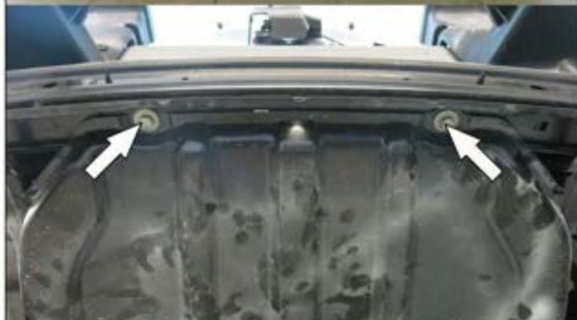
12. Remove 2 bolts out of skid plate fitting.
