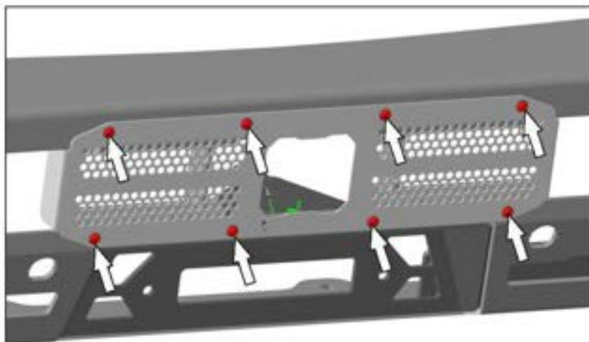
32. Install decorative pad (13), using screws M6x25 (G), washers 6 (M), nuts M6 (J), as shown.
