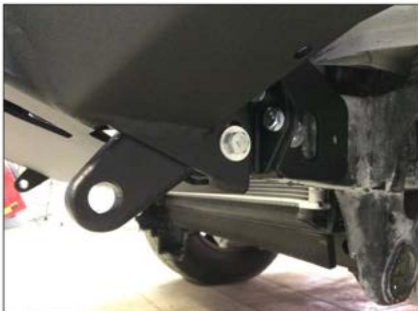
37. Install bumper body (1) onto the winch bracket (2). Fix its lower part to brackets using bolts M10x30 (D), insert nuts M10 (T) and washers 10 (P).
