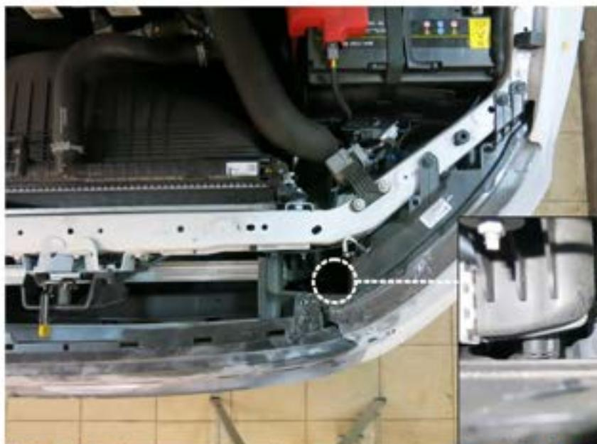
8. Remove 2 bolts out of lower part of radiator grill, then remove radiator grill.
