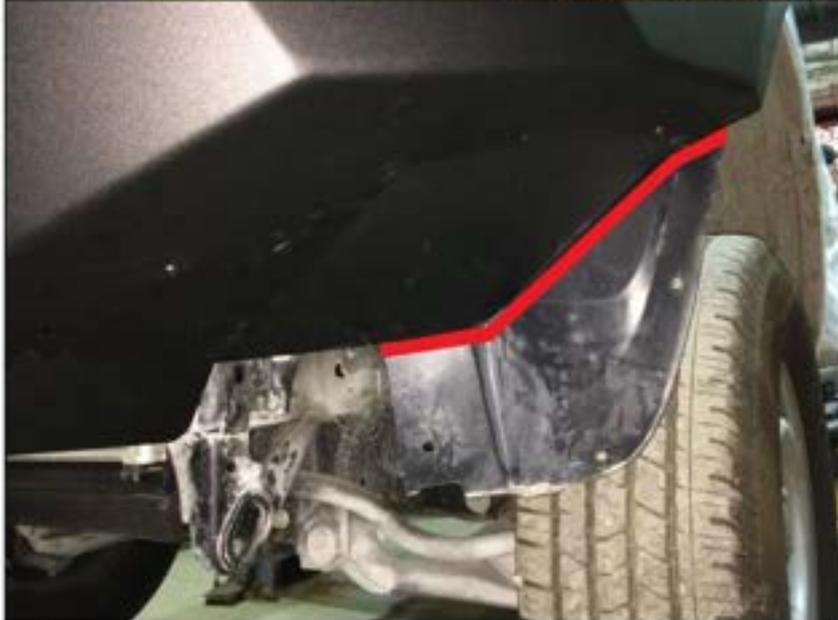
44. Push the flaps (7, 8) to OE plastic fenders and mark the cut line, then cut OE plastic fender.
