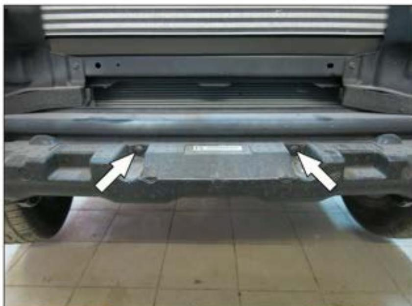
11. Remove plastic plugs out of the panel. Remove the panel.
