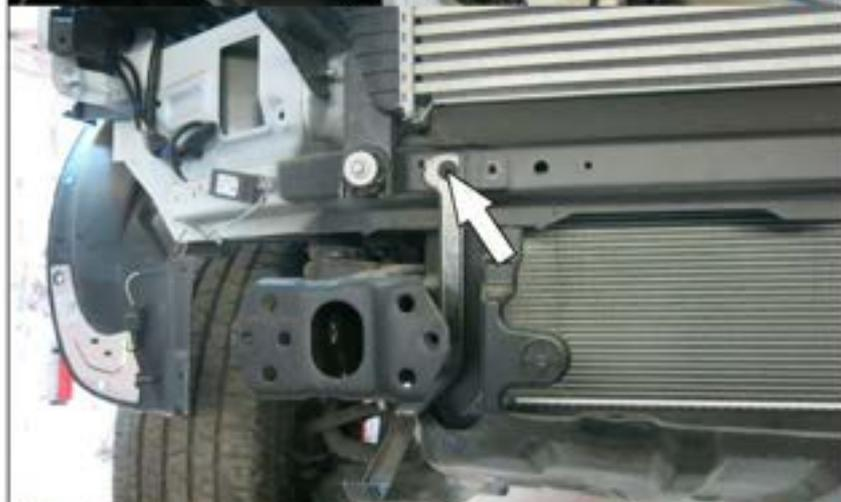
16. Remove the bolts, then remove the bumper panels.
