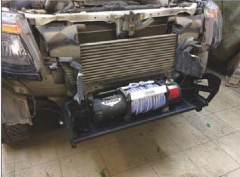
26. Place the winch to the bracket (2), and fix it with the bolts supplied with winch.
