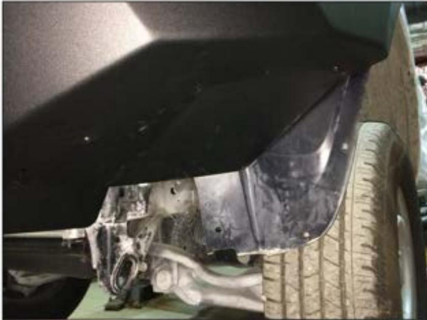
43. Install flaps (7, 8) using screw M6x20 (F) and washers 6 (M). Make sure the flaps are fixed inside of the bumper, not outside.
