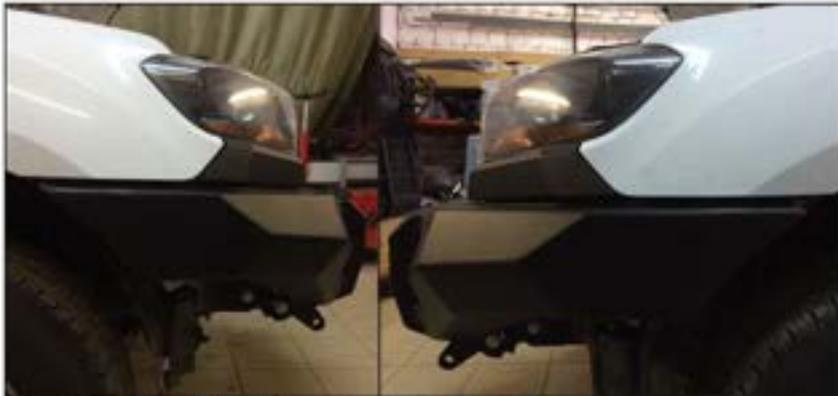
39. Adjust bumper until you have an equal gap between vehicle body and the bumper on both sides. Tighten bolts after that.
