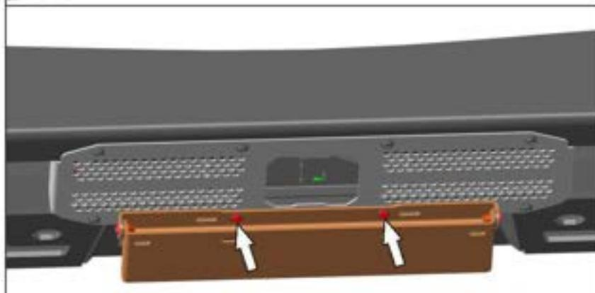
33. Install license plate (4) using screws M6x25 (G), nuts M6 (J) and washers 6 (M).
