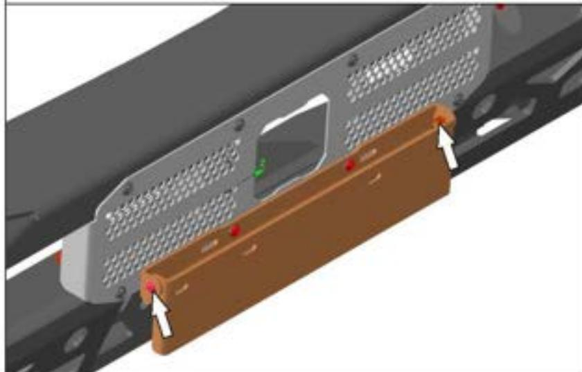
34. Adjust the angle of license plate. Tighten all connectors after that.
