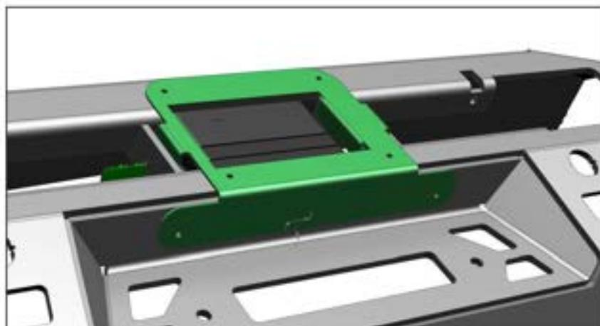
28. Install template (16), as shown. Mark the shape of cut out and prick 6 holes.
