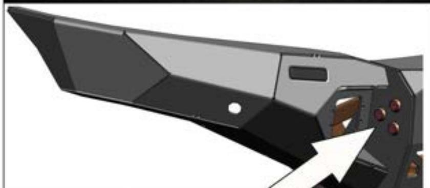
38. Place screw M10x30 (H) with countersunk washers (S) from both left and right sides as shown on the picture and secure with nuts M10 (L) and washers 10 (P).
