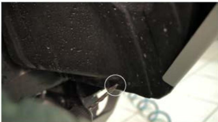
45. Mark a hole from inner side of the wheel fender from both left and right side of vehicle. Drill a 6-8 mm diameter hole.
