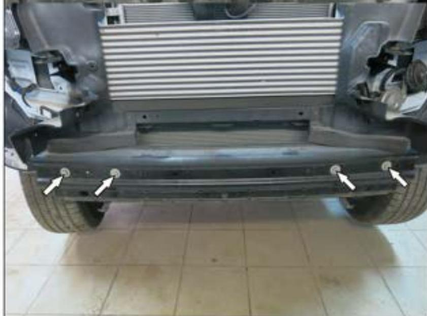
13. Remove 4 bolts out of front bumper bracket. Remove the bracket.
