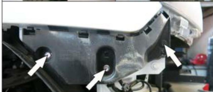
15. Remove 3 bolts out of plastic brackets from both left and right sides of the vehicle.
