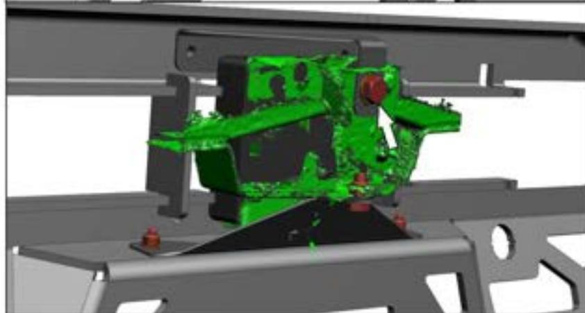
31. Fix the bottom part of radar using bracket №1 (14), bolt M10x20 (C), washers 10 (P) and nuts M10 (L), as shown.
