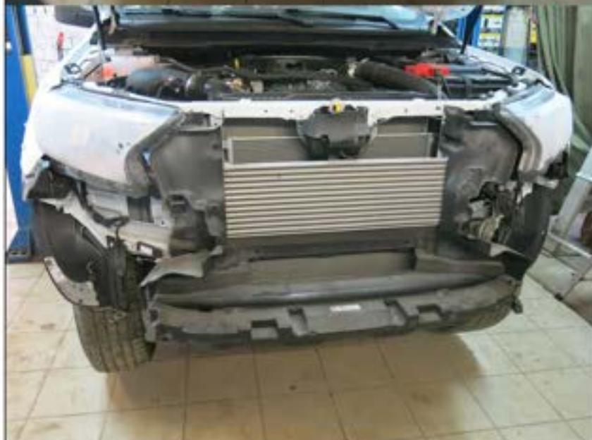
10. Remove the bumper by pulling the bumper towards you holding the sides.
