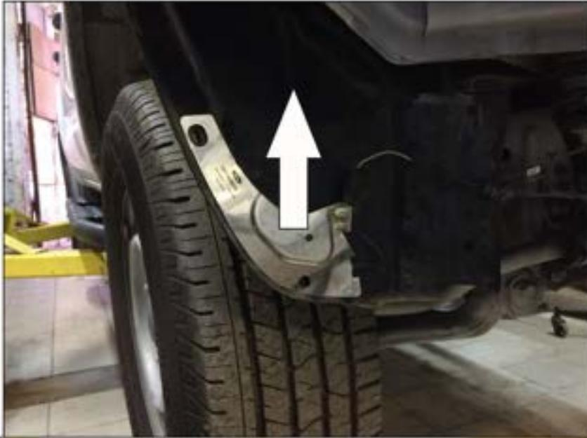
41. From right side, unstick antenna from the fender. Move antenna upper under the bar.
