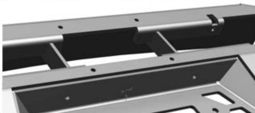
29. Cut the hole in bumper out, by follow the marked line
