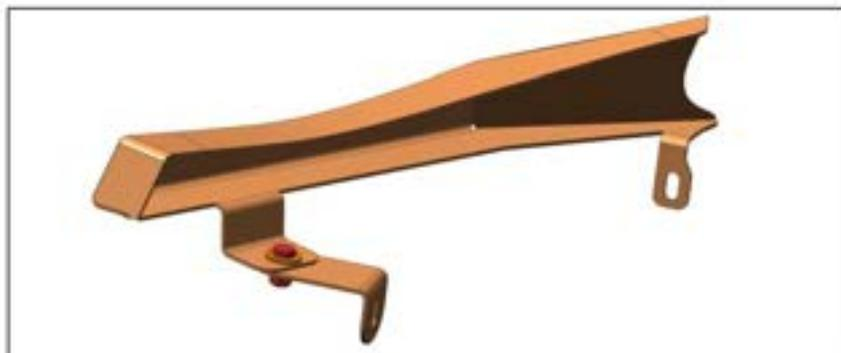
17. Mount bracket (17) to panels (11, 12) as shown on the picture. Fix them with bolts M6x20 (A), nuts M6 (J) and washers penny 6 (N).
