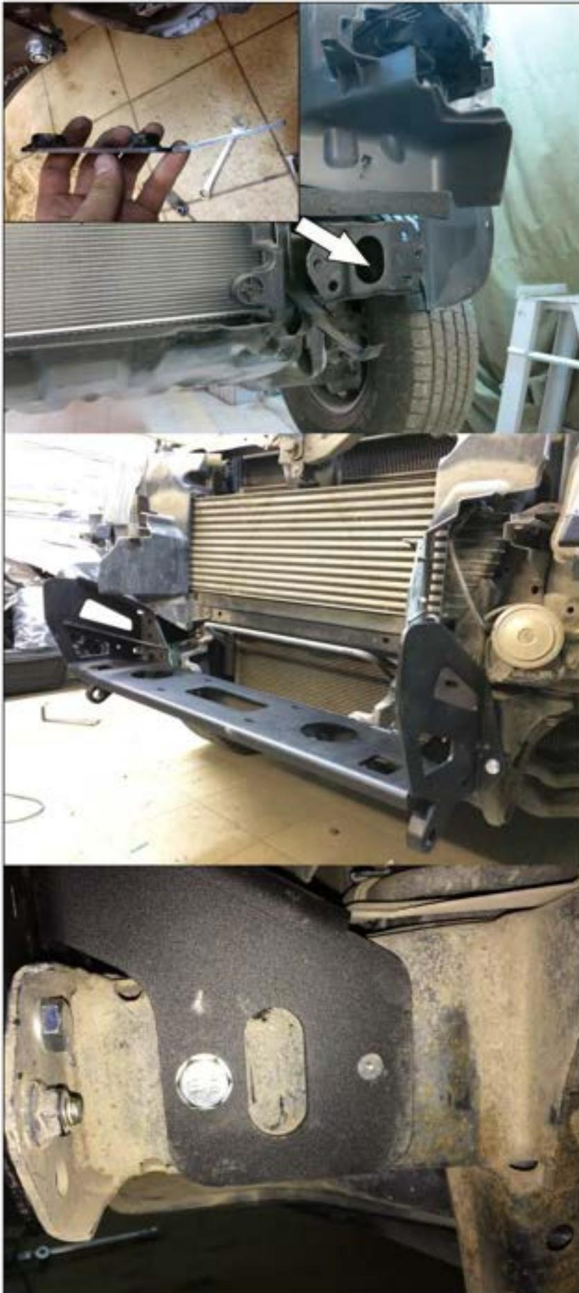
22. Place insert nuts (U) into the chassis.
