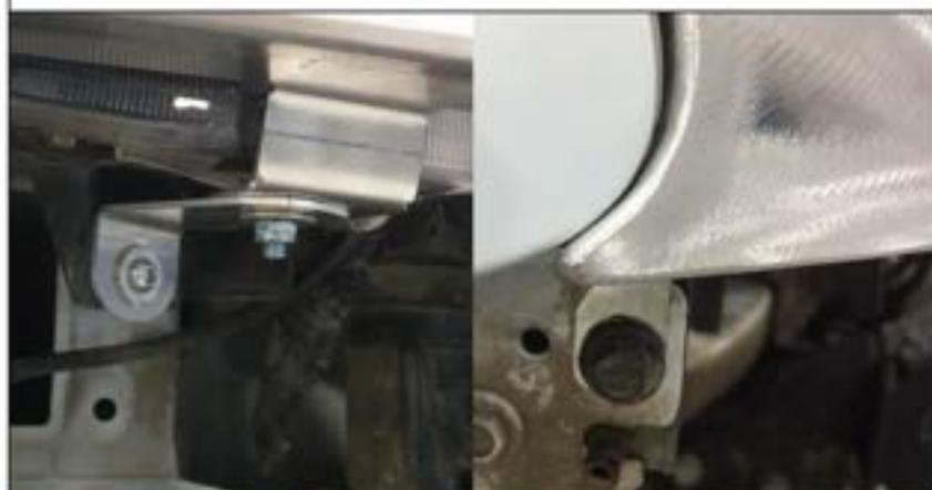
18. Install panel under headlight. Fix bracket under headlight. Fix them with screw M6x20 (F) and washers penny 6 (N).
