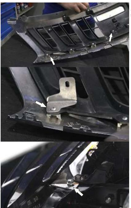
55. Unscrew specified screws on each side of the radiator grill.
