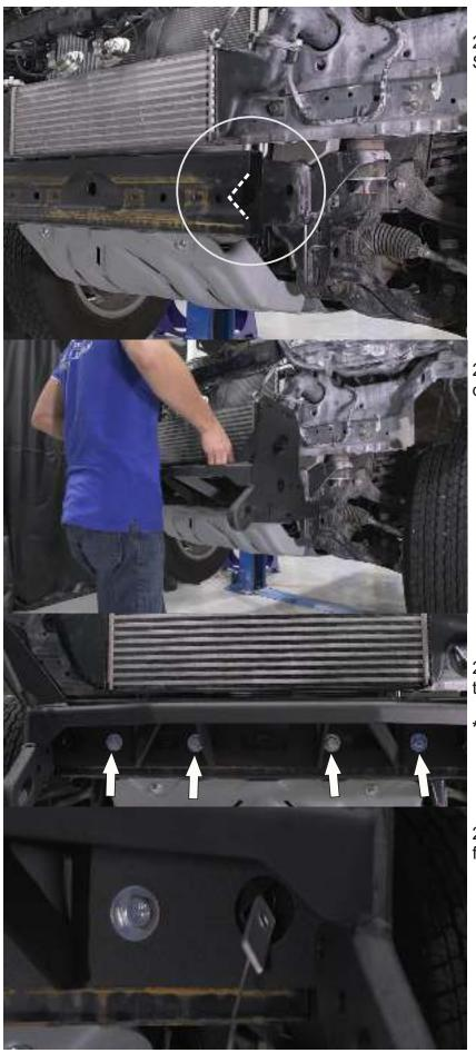
23. Make cutouts in the safety beam. Scarf and paint all trimming points.
