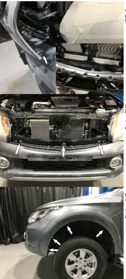
4. Dismantle the radiator grill. Carefully pull the grill edge by unlatching the latches.
