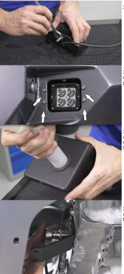
36. Install lights onto the brackets.
