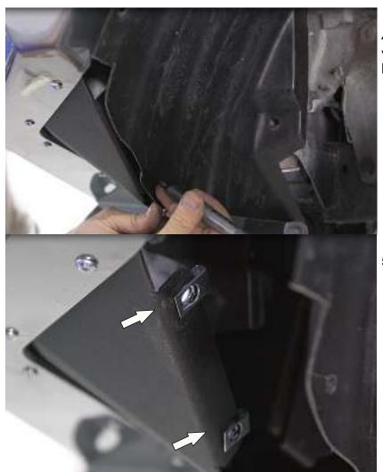
49. Install the mudguard onto the vehicle, mark drilling points opposite the holes of the flap and drill the flap holes.
