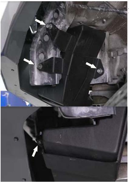
40. Install the washer reservoir using the bracket and standard fittings.
