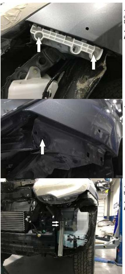
14. Unscrew bolt and self-tapping screw of the plastic clamper. Dismantle the clamp.
