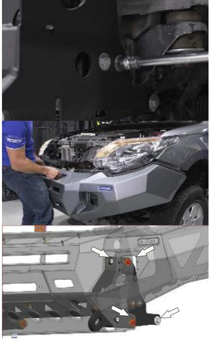
31. Tighten all screw joints of the bracket to the vehicle frame.
