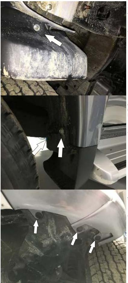
7. Unscrew the splash guard self-tapping screw
