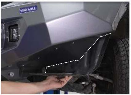
47. Install mudguards onto the vehicle and mark the cutting line.
