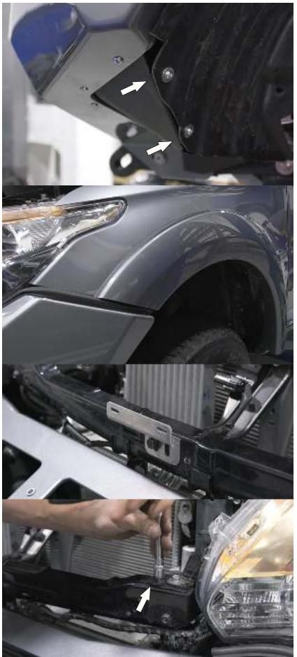
51. Secure mudguards to the flaps using screws M6x20 and washers.
