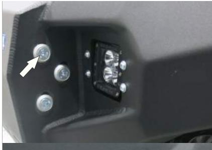
44. Fix bracket and bumper body through drilled hole using screws M10x30, nuts M10, countersunk washers 10, washers 10.
