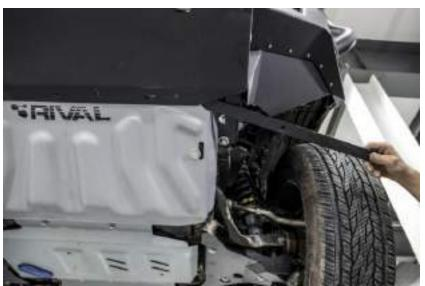
53. \*Fix underbody armour to the bumper body using insude nuts, screws M10x30 and inside washers.
