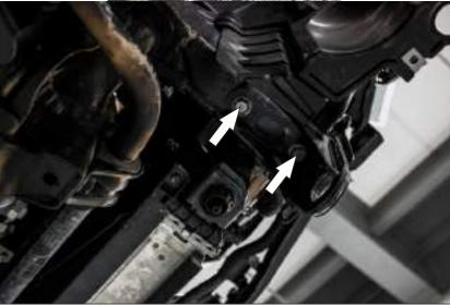
20. Remove 2 bolts. Remove OE towing hook.
