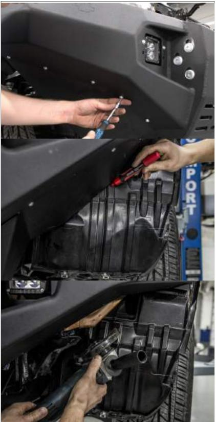
47. Mount flaps on bumper using screws M6x20 and washers 6.
