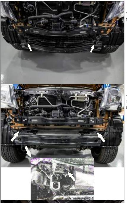
18. Remove caps of air intake mount. Remove air intake.
