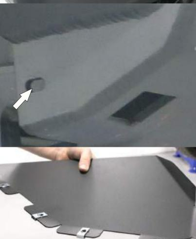
45. Drill 10mm holes in lower part of bracket through drilled holes. Mount bumper body on bracket using screws M10x30, nuts M10, countersunk washers 10, washers 10.
