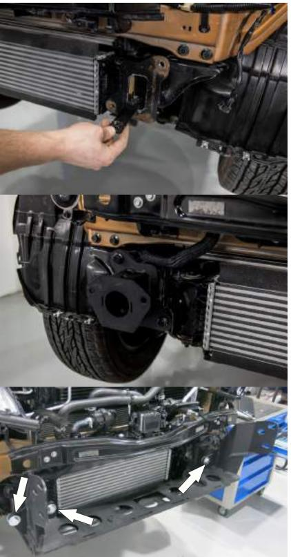
29. Mount inside nut M12x1,25(11) into the chassis from the left side of vehicle.
