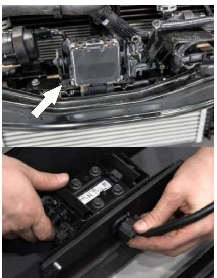
\*For vehicles with radar 35. Remove radar.
