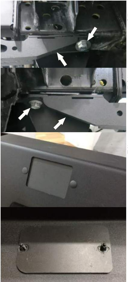
32. Mount lower part of bracket from the left side using bolts M12x1,25x40 and washers 12.
