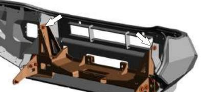
27. Mount bumper body onto the winch bracket using bolts M10x30 (17), washers M10x30 (30) and nuts M10 (26).
