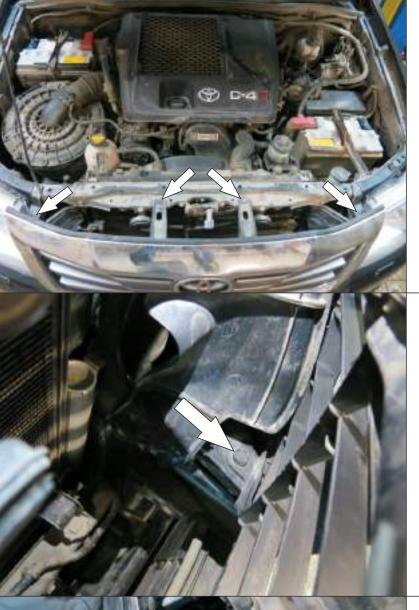
1. Open the bonnet and remove all scrivets holding the grill in place.
