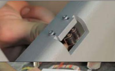
23. Mount roll latches (32) to bumper (1) with screws M3x12 (20) and nuts M3 (24).
