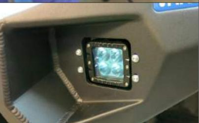
33. \*Install brackets with LED lights using bolts M6x16 (21) and washers M6x12 (27). Adjust the LED position.
