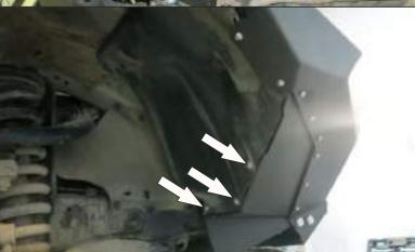
40. Mark drill points on plastic fenders in accordance with the apertures in the flaps. Using a 6-7 mm drill bit, drill holes.
