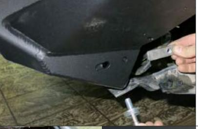
28. Place insert nut plate M10 (11) as shown. Screw blind-head bolt M10x35 (23) with countersunk washer.
