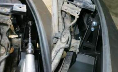
31. Using a 10mm drill bit, drill into the hole through the existing hole of the winch bracket from both left and right. This is to increase the size of the existing hole.
