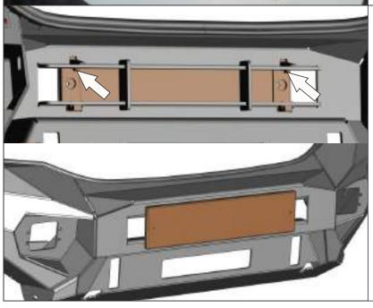
25. Place license plate holder on the bumper, fix it with bolts M6x16 (15). Adjust latches horizontally and vertically until in desired position. Tighten all screws.
