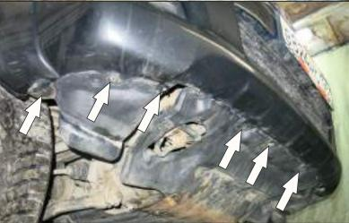
5. Remove lower bumper retaining screws.
