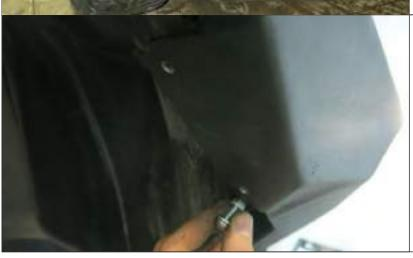
37. Using a 6-7 mm drill bit drill holes in plastic fender in accordance with holes in flap. Fix flaps with bolts M6x20 (22), washers M6x12 (27) and nuts M6 (33).
