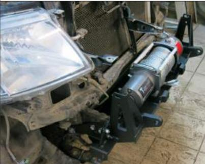
21. Mount the winch (not supplied) following the winch installation instructions supplied with the winch manufacturers.
