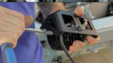
32. \* Mount LED lights into brackets (6). Adjust and tighten them.
