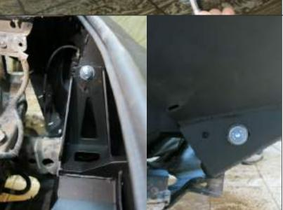
29. Adjust bumper so that there is an equal gap between the bumper and the vehicle body on both sides.
