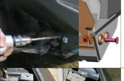
30. Using a 10mm drill bit drill a hole through the bumper body and the winch bracket from both left and right.
