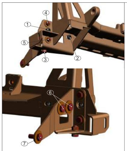
20. Align winch bracket horizontally and vertically.
