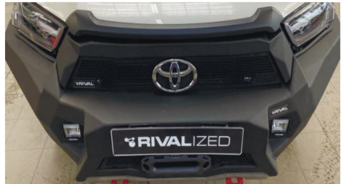
64. Install the emblem badge on grill surface (pos.2). Install grill (pos.2) on brackets (pos. 12-15), using screw M6x20 (pos. G) and washer 6mm (pos. L).
