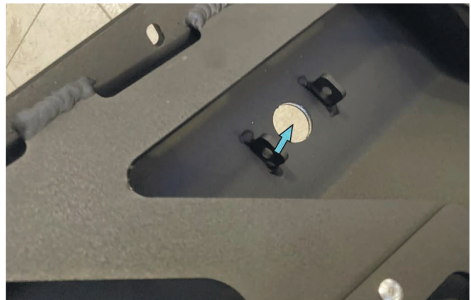
28. Locate knock-outs for parking sensors on the bumper body (pos.1) and knock them out by a hammer.
