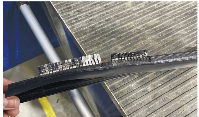
40. Bend the reinforcement of the seal where cut.
