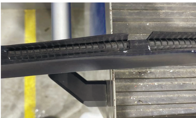
41. Remove the reinforced section of the seal.
