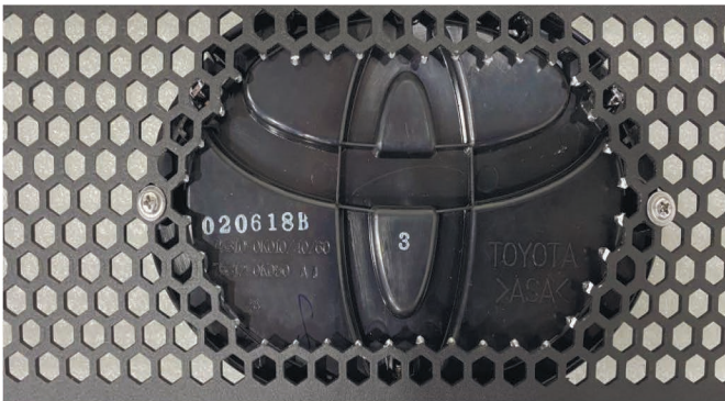
69. Make a cutout, then trim the sharp edges and mounts the emblem badge.
