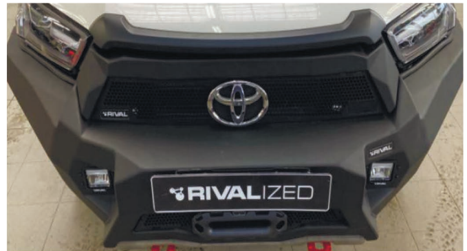
70. Install the emblem badge on grill surface (pos.2). Install grill (pos.2) on brackets (pos. 12-15), using screw M6x20 (pos. G) and washer 6mm (pos. L).
