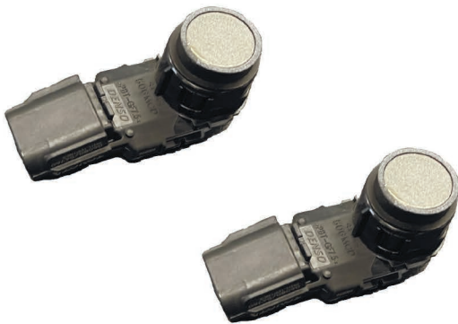
27. Remove parking sensors from factory bumper.
