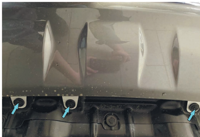
9. Remove the screws securing the lower center part of the bumper.
