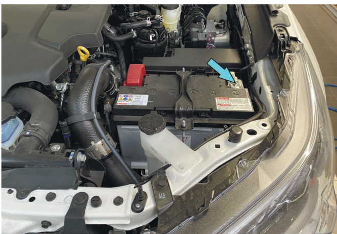
71. Connect terminal "-" of the battery.
