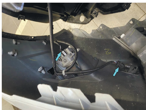
11. Disconnect the connectors of the fog lights and parking sensors.
