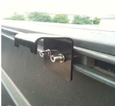
*\*Line the bracket up with the tri-fold hard cover clamp location once they are lined up. Secure bracket to the vehicle bed rail.*
