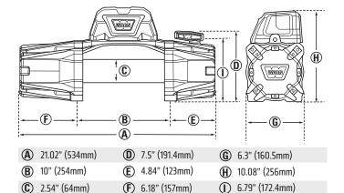
**Winch Dimensions:** 21" L x 6.3" D x 10.1" H (534mm L x 160.5mm D x 256mm H)
